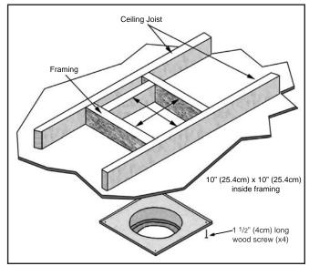
Figure 33: Wall Framing for Hole for Vertical Installation.
