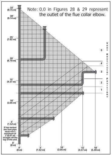
Figure 28. Possible Vent Configurations for Top Vented; Vertical and Horizontal Terminations.
