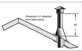
Figure 36: Height of Vertical Termination;
