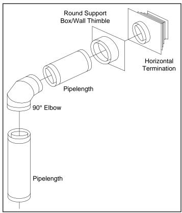
Figure 24: Common Horizontal Installation.
