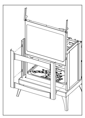
Figure 18: Removal of Door and Fascia.
