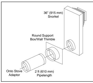
Figure 26: Common Snorkel Installation.
