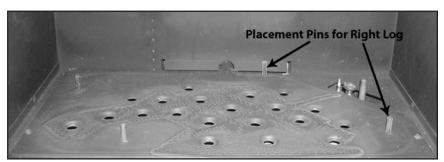
Figure 59: Step 1 of Log Placement.
