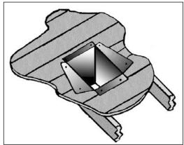
Figure 40: Cathedral Ceiling Support Box Installation.
