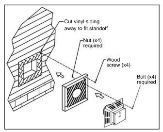
Figure 32: Installing Vent Cap with Vinyl Siding Stand-Off.
