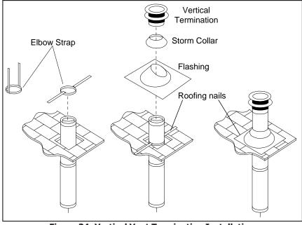
Figure 34: Vertical Vent Termination Installation.
