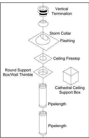
**Figure 25: Common Vertical Installation.**
