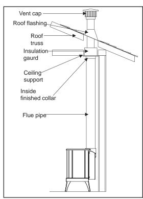
Figure 48: Installation for Top Vented; Vertical Termination.
