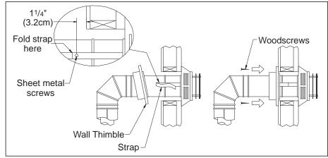
Figure 31: Installing Decorative Wall Thimble.
