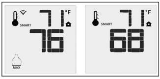
Figure 10: Remote Control's Smart Flame Function.
