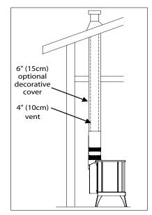
Figure 52: Unit top venting styles.
