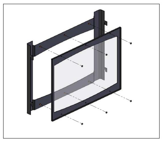
Figure 71: Safety Screen Removal
