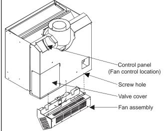
Figure 58: Optional Fan Kit Installation.
