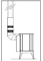
Figure 53: Unit rear venting style.
