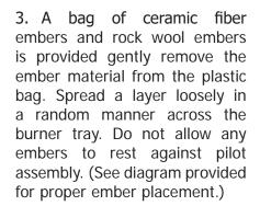
DO NOT pack this ember material as this could create an unsafe condition, leave embers loose.
