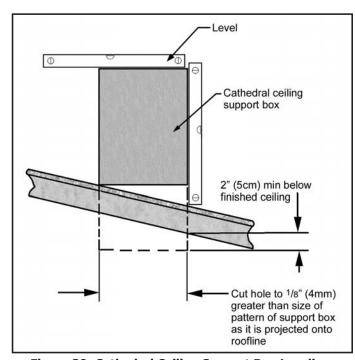
Figure 39: Cathedral Ceiling Support Box Leveling.
