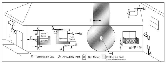
Figure 26. Vent Termination Restrictions, refer to Table 3.
