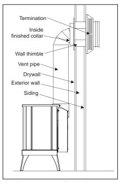
Figure 47: Installation for Top Vented; Horizontal Termination.
