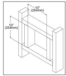
Figure 30: Wall Framing Hole for Horizontal Installation.
