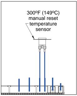
Figure 51: Spill Switch Wiring Diagram
