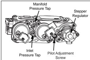
Figure 56: Fully Labeled Gas Valve.
