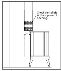
Figure 54: Draft test place.
