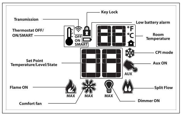
Figure 5: Proflame 2 Transmitter LCD Screen.
