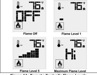
Figure 11: Remote Control's Flame Levels.
