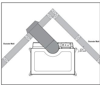
Figure 42: Corner installation top vented.
